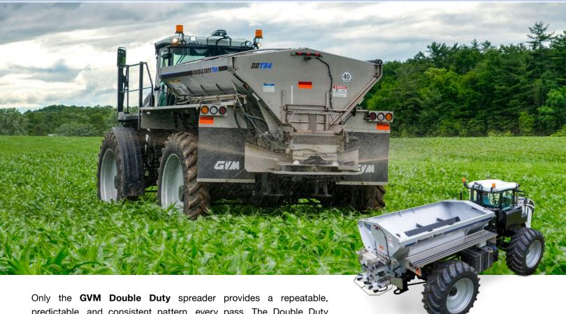
predictable, and consistent pattern, every pass. The Double Duty spreads a guaranteed flat, 90- to 105-foot pattern without timeconsuming spinner or funnel/chute adjustments between materials or rates. A 120-foot pattern can be achieved with some materials. Pinpoint product control and its widespread pattern allow the Double Duty to spread more acres annually with less compaction, less fuel, and fewer stops to maximize your productivity and profitability.
