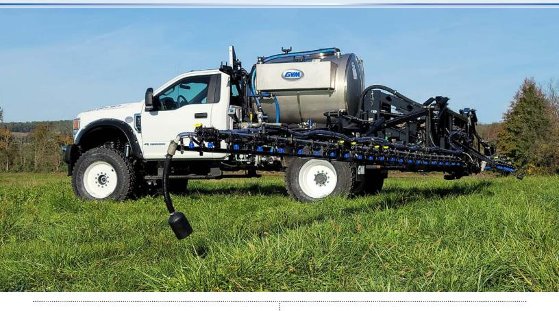
The GVM Hydra Spray was designed to offer versatility and maneuverability to custom applicators, co-ops and farmers. The Hydra Spray is offered from the factory on the Ford F-550 chassis. This provides operators a narrow, mechanical drive machine with a tight turning radius and comfortable road travel.
