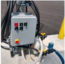
GVM's Overhead Spray Systems (OSS) are multifunction liquid deicer dispensing systems designed to pre-wet truck loads of solid de-icing materials. Pedestal Pre-Wet Systems allow users to pre-wet multiple truckloads with only one dispensing system. Pedestal systems are also capable of loading and unloading truck-mounted pre-wet tanks, returning the de-icing liquids to bulk storage tanks, and draining tanks for end-of-season maintenance.
