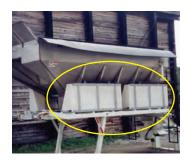
width to the body. This system can be set up for single or dual tank application. When dual tank application is utilized, the tanks are plumbed together, allowing solution to be evenly drawn from each tank, to maintain an even weight distribution. V-Box mounted systems are available in 30, 60, 70, 100, 140, 200, 280, 400, and 450 gallon sizes, and with the dual tank option, offers a maximum 450 gallon capacity.
