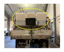
signed for quick installation and removal from the tailgate. The carrier uses four pull-pins and a lifting eye to facility ease of system installation and/or removal. Tailgate mounted system are available in 30, 70, 100, and 135 gallon sizes.
