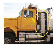
the side of the dump body or between the cab and dump body. Chassis mounted systems are available in 60, 90, 120, and 240 gallon sizes.
