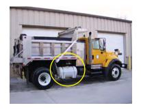
on the side of the dump body. Frame mounted systems are available in 35, 55, 65, and 100 gallon sizes.
